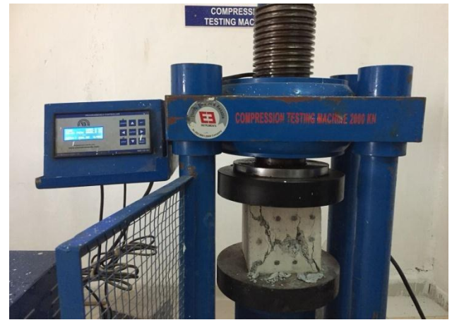
Development of Cracks
