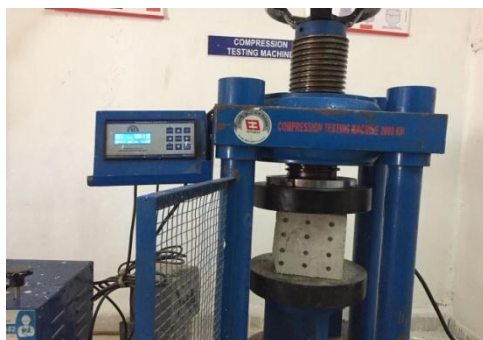
Testing of Blocks
